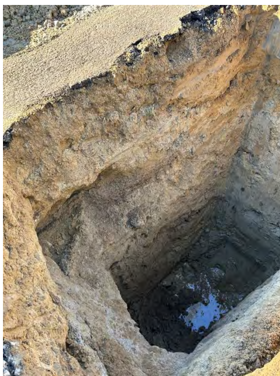
Photo 2: Test Pit TP-01 Sidewall
